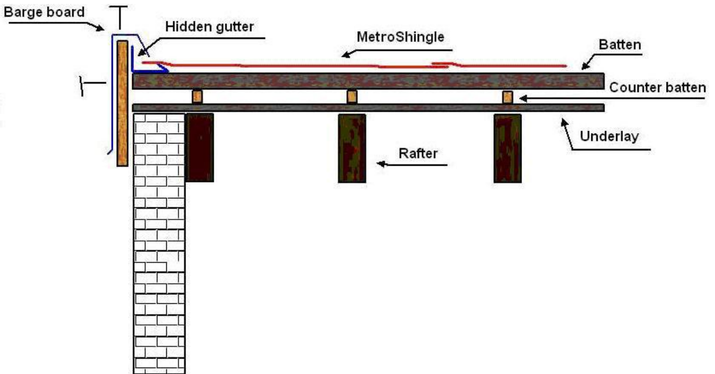
Figure 4a Roof edge Metro Shingle
