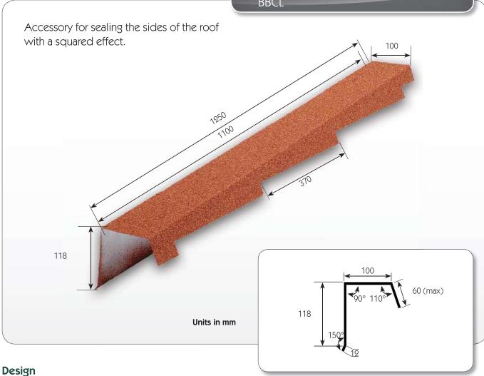
The barge board cover is designed to give your roof a squared 'finishing' effect.
