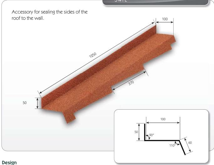
The lefttsided wall flashing is designed to make a nice finish between your roof and the wall that is next to it.
