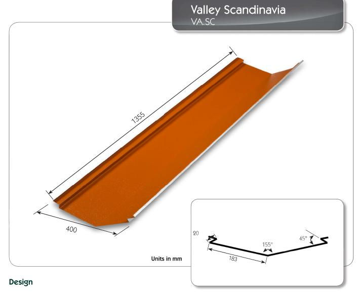
A roof valley plagna is designed area where two adjacent roof sections meet, usually at a 90-degree angle. Water runoff funnels into this valley from both roof sections.
